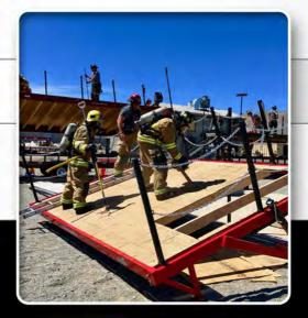
FireVent's Portable Units are designed to be easy to set up and take down and move from location to location. These units are able to go from a flat position to a 12/12 pitch. There are currently two sizes available; 8ft x 12ft and 10ft x 16ft.
