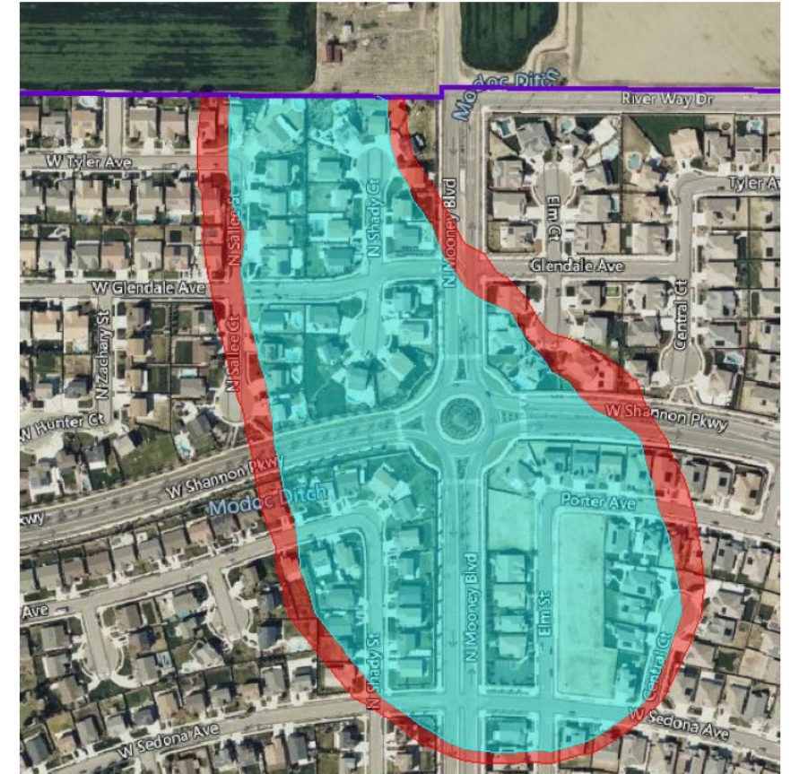
Figure 4: Example Inset of an Area Spared from Flooding by the 100- Year Flood near the St. Johns River along the North Edge of Visalia. Areas subject to flooding by the 100- year post-condition flood shown in blue. Additional areas subject to flooding by the 100- year pre-condition flood but not the 100- year post-condition flood shown in red. Visalia city limits shown in purple.
