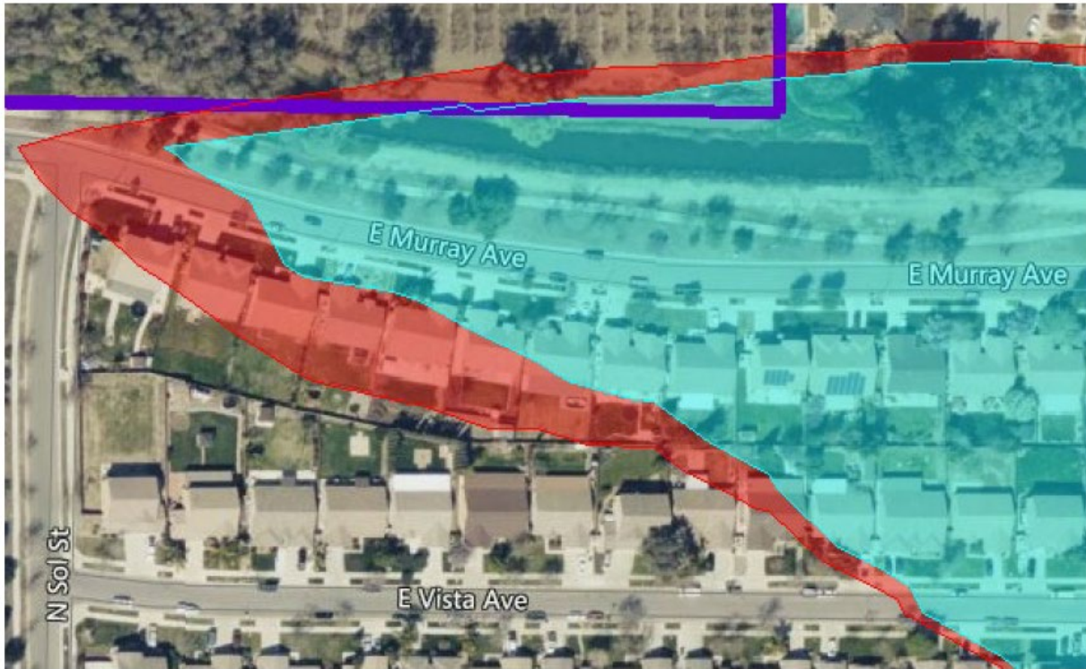
Figure 3: Example Inset of an Area Spared from Flooding by the 100- Year Flood along Mill Creek near the East Edge of Visalia. Areas subject to flooding by the 100- year post-condition flood shown in blue. Additional areas subject to flooding by the 100- year pre-condition flood but not the 100- year post-condition flood shown in red. Visalia city limits shown in purple.
