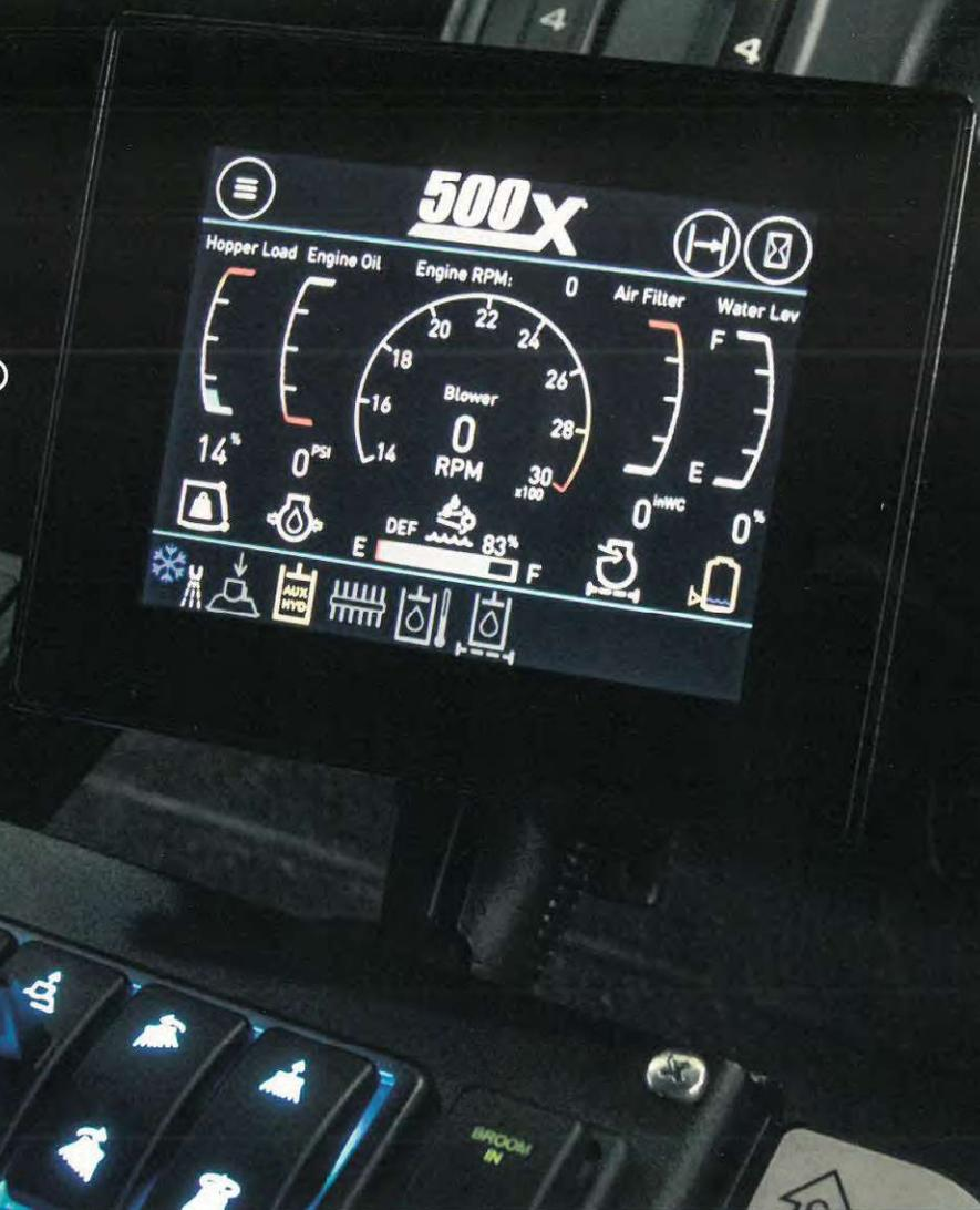
**TYMCO, the inventor of the Regenerative Air System, delivers industry-leading technology with its BlueLogic Control System! BlueLogic is the sweeper multiplex electronics system that controls sweeper functions as well as provides On-Board Diagnostics (OBD). The BlueLogic Display provides valuable information including: hour meters, operational messages, service reminders, event logs and sweeper statistics such as fuel usage, water usage, and sweeping mileage.**
