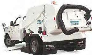
Model 210/300 – More compact, highly maneuverable sweepers designed specifically for use around parking and maintenance areas, airport roads, hangars, and low clearance terminal areas (such as passenger air bridges).
