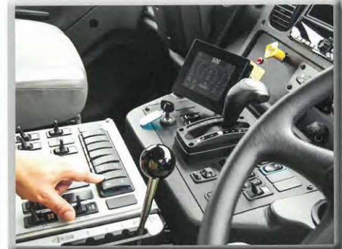
**OBD for Auxiliary Engine and Sweeper:** The in-cab display delivers code reader functionality by providing fault information for the auxiliary engine and sweeper via detailed on-screen messages when a fault is active. Active auxiliary engine and sweeper faults can also be viewed on Status Pages within the BlueLogic Display.
